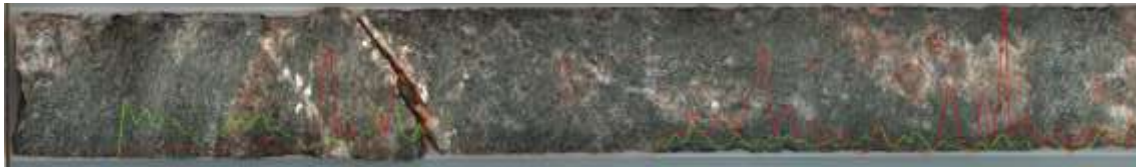
The variation of Endialyt (green) and Catapleiite (red) along the core
