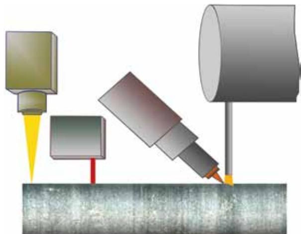
*This image shows the schematic setup for qXRF, with from right x-ray tube, XRF detector, distance meter and camera.*
