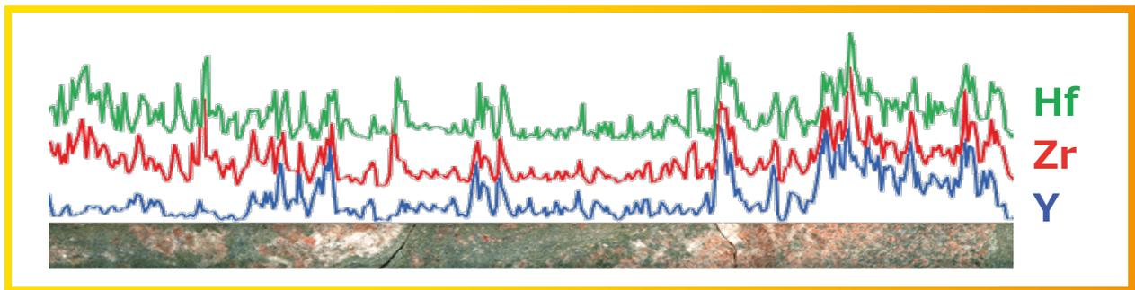
In this image is shown a photo of a core from Norra Kärr REE mineralization, Sweden, together with graphs displaying the variation of Hafnium (Hf), Zirconium (Zr) and Yttrium (Y) along the core. The average concentrations for these elements are  $Y \sim 0,19\%$ ,  $Zr \sim 1,21\%$  and  $Hf \sim 0,05\%$ . Another 26 elements were determined simultaneously. This scan was performed using one millimeter steps.
