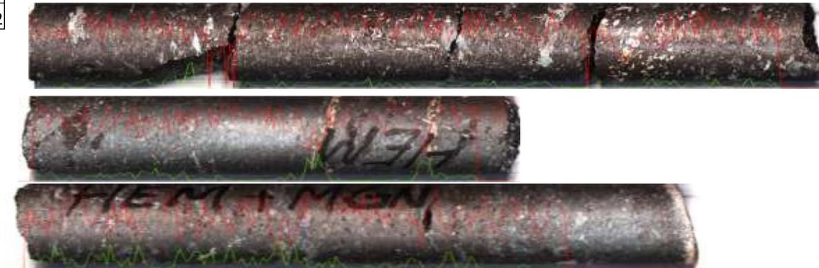
The elemental profile of Ca (green) and Fe (red) along the three core sections core in 1 mm resolution.
